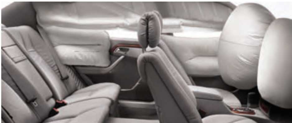
Air bag illustration showing full deployment of all air bags, shown in an S-Class Sedan
