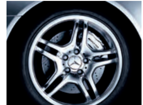
E55 AMG perforated front brake and 8-piston caliper
