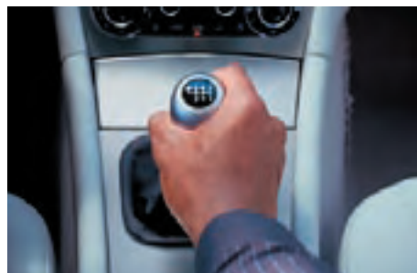
6-speed manual short-throw gearshift
