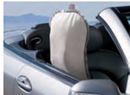
Head-thorax side air bag, shown in a CLK-Class Cabriolet
