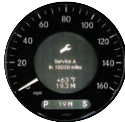
Multifunction display: Maintenance System
