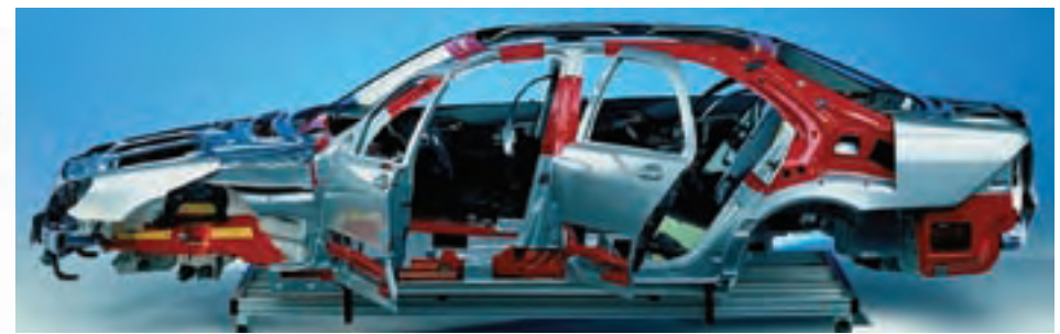
Typical Mercedes-Benz body structure (S-Class sedan shown)
