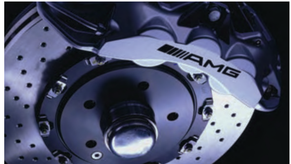
SLK55 AMG compound, perforated front brake and 6-piston caliper
