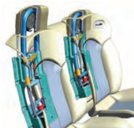
CLK-Class Cabriolet pop-up roll bar components
