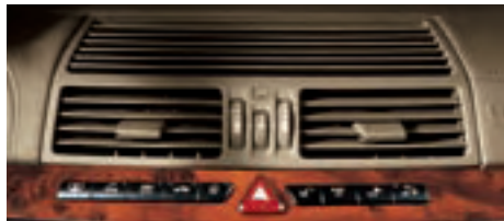
High-flow/low-draft air outlets shown in an S 600
