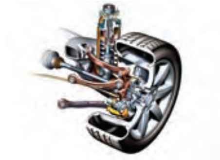
Multilink rear suspension (SL 500 shown)
