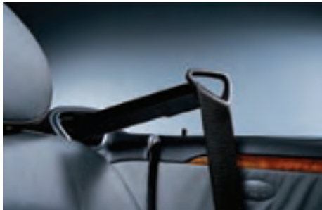
CLK-Class Coupe automatic front seat-belt presenter
